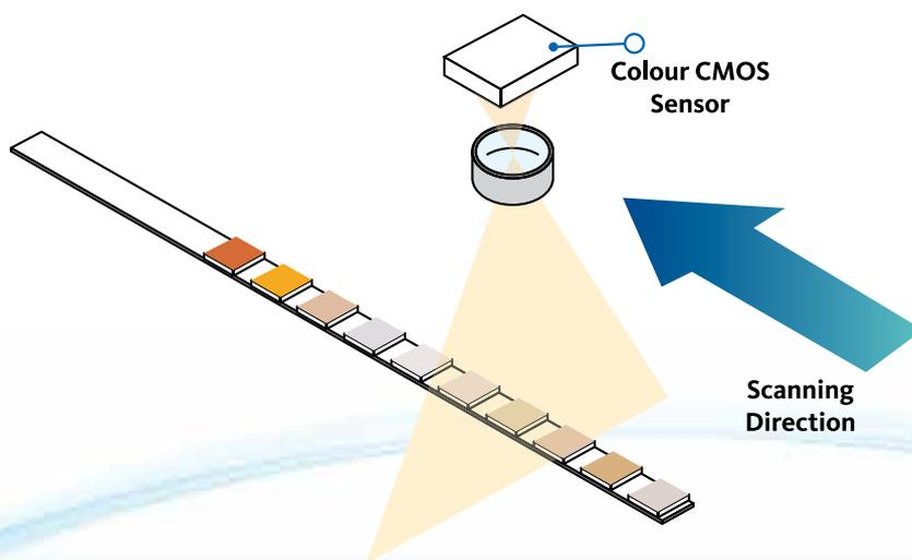
Photometry is performed with smart CMOS sensor image enabling high-accuracy measurement.
