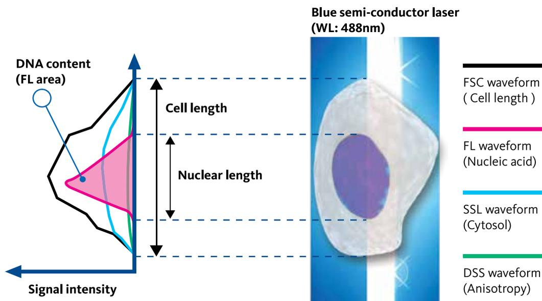
FSC, FL, SSL and DSS scattergrams are automatically generated to recognise specific and unique properties of different particles by size, labeling DNA, complexity and specific features, and so determining the particle type.
