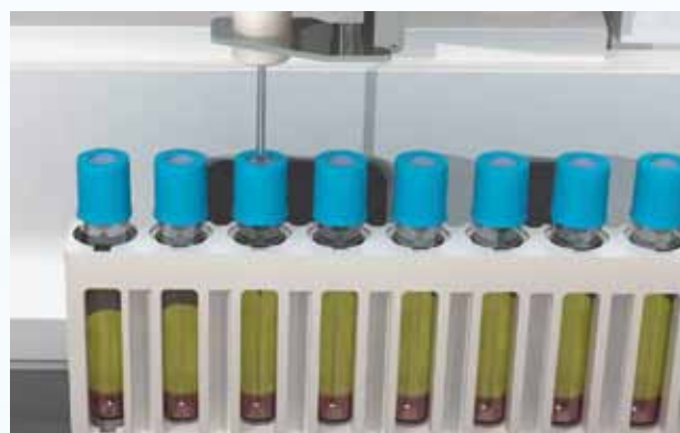
Cap-piercing on CS-2500 *CS-2400 is a non cap-piercing model
