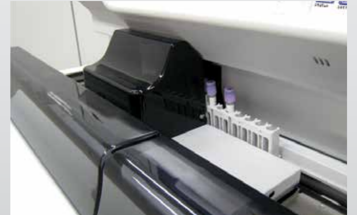
Smear preparation and cell pre-classification based on user-defined rules and sample condition
